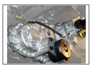
4. Pull the shift motor assembly out while keeping the level. Clean the mating surface of the transfer case and shift motor.
