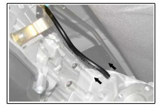
3. Disconnect the air hose from the transfer case.
