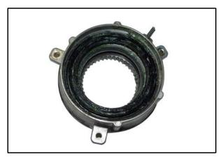
Check the internal seal ring of hub actuator for damage.
