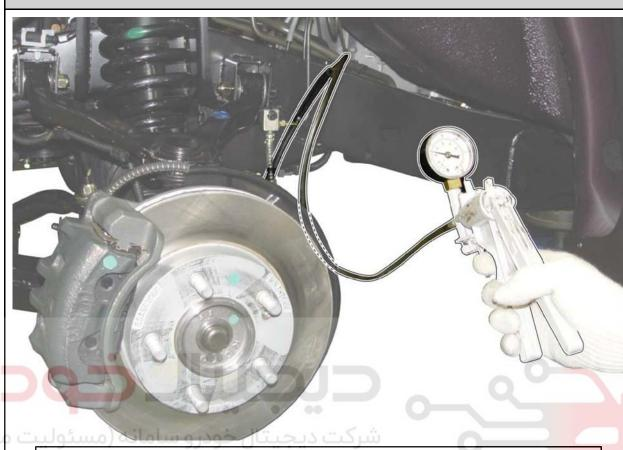
Disconnect the vacuum hose from the hub actuator and install the vacuum pressure gauge to the hub actuator. Apply vacuum pressure to make sure the hub actuator maintains vacuum pressure.
