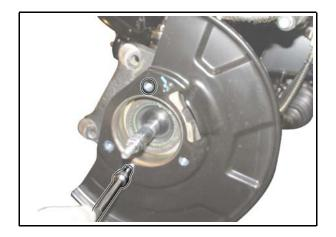
1. Unscrew the two bolts (10 mm) and remove the brake dust cover.
