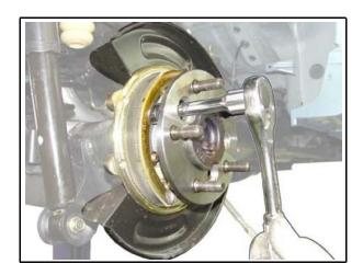
7. Unscrew the four flange lock bolts (17 mm) on the axle housing flange and remove the axle shaft.
