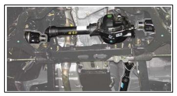
2. Removal of mounting bolt Unscrew the mounting nut (22 mm) at right side of the axle housing and remove the axle mounting bolt.
