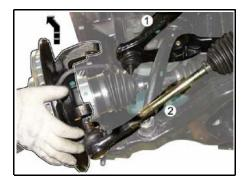
3 Loosen the upper arm (1) and the tie rod end (2) and remove the assembly by lifting it.
