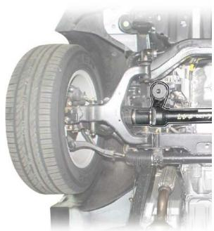
3. Unscrew the four bolts (17 mm) on the axle housing and remove the axle mounting bracket.
