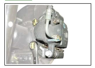
1 Unscrew the two mounting bolts (19 mm) and remove the rear brake disc caliper. Secure the removed caliper on the vehicle frame.
