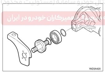
Remove the bearing fixing snap ring of inner shaft and pull off the bearing. Remove the inner shaft and housing bracket
