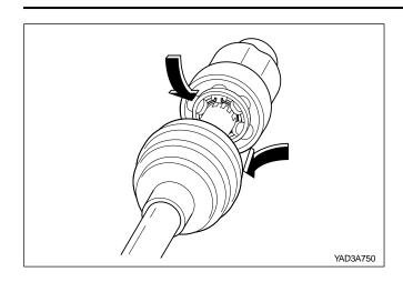
3. Apply the specified grease to the joint housing.
