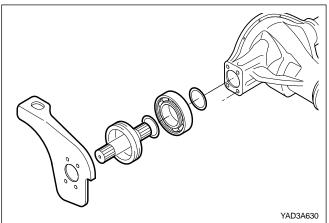
8. Assemble the parts of the front axle inner shaft and housing mounting bracket.
