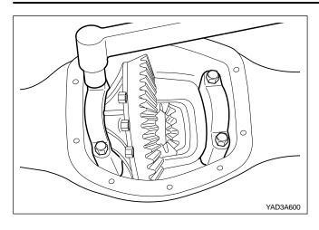
5. Install the differential carrier assembly into the axle housing. Set up the bearing cap and then tighten the cap bolts.
