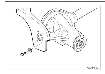
9. Align the axle shaft and differential carrier spline and insert the axle shaft. Assemble the axle housing mowiting bracket to the axle housing.
