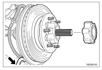
• Detach the vacuum hose of locking hub from steering knuckle.
