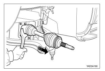
11. Remove the drive shaft using the special tool.
