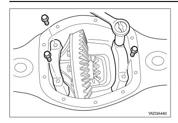
Remove the bearing cap mounting bolt and pull off the bearing cap. Pull out the differential carrier assembly.
