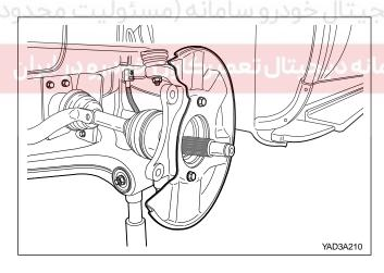
4. Install the dust shield to the knuckle.
