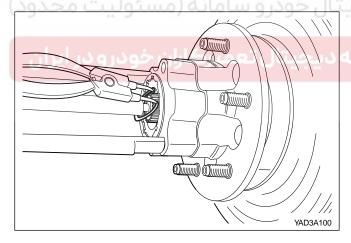
Remove the retainer ring & outer shin in the drive shaft and pull off the lock.
