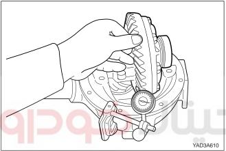
6. Measure the backlash of drive pinion and ring gear.
