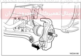
10. Carefully remove the steering knuckle assembly.
