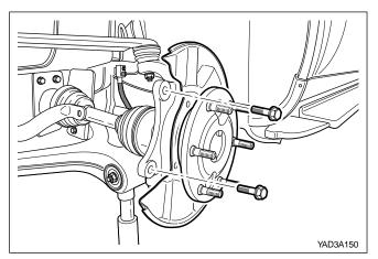
Remove three wheel bearing bolts (M12) and pull off hub assembly by using the special tool.
