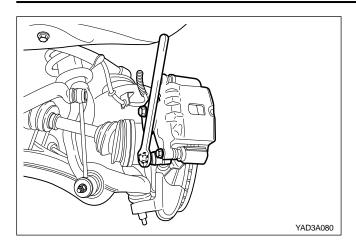
Remove the two knuckle-brake caliper assembly mounting blots and pull off the caliper assembly.
