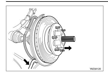
• Remove the hub & brake disc assembly.
