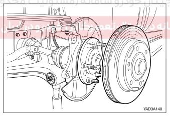
Remove the front disc assembly from the axle shaft.
