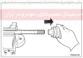
5. Remove the drive axle shaft.
