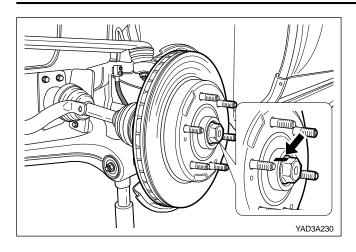
Install the front disc and tighten the hub nut & washer. When you install then, align the hub nut-washer to the shaft end and tighten the hub nut as the specified torque. After bending the groove part of shaft, apply the painting and grease to the groove part.
