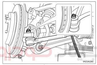
8. Insert the steering linkage ends to the steering knuckle and tighten the slot nut.
