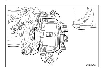
7. Tighten the front disc brake caliper assembly mounting bolts on condition that the front disc is mounted.
