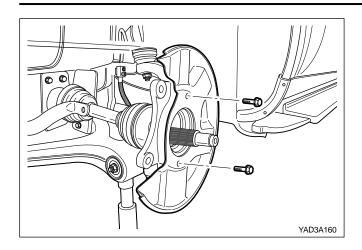
7. Remove two dust shield mounting bolts (M6) and pull off the dust shield.
