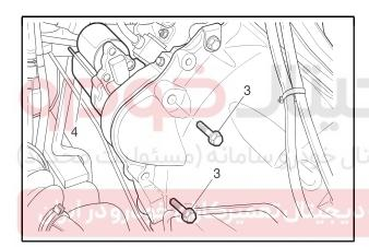
4. Unscrew the mounting bolts (3) of starter.
