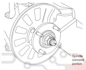
Installation of the rear speed sensor (For vehicles equipped with ABS(Anti-lock Brake System)): Insert a feeler gauge into the space between the pole piece of the speed sensors and the rotor teeth surface, and then tighten the speed sensors at the position where the clearance at all places is within the standard value.
