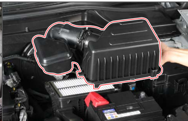
Remove the air cleaner upper cover mountings to remove the air duct hose with the air cleaner upper cover.
