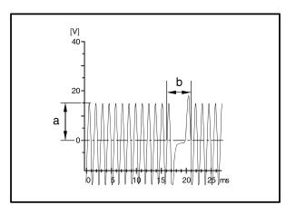
Measure the output wave between the ECM terminals No. 99 and No. 100 using the scan tool or the oscilloscope while engine cranking (start motor activated).
