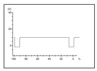
1. Measure the output wave between the ECM terminals No. 104 and No. 106 using the scan tool or the oscilloscope while engine speed is at idle.
