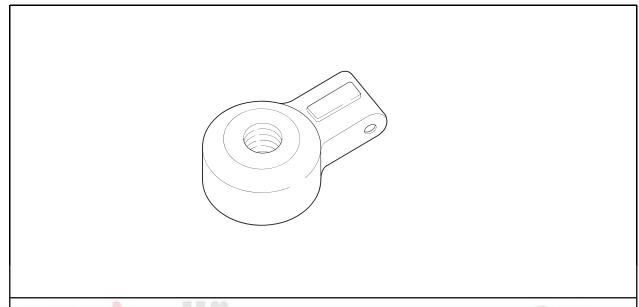
The Knock Sensor (KS) detects abnormal knocking in the engine. The two KS are mounted in the engine block near the cylinders. The sensors produce an output voltage which increases with the severity of the knock. This signal is sent to the Engine Control Module (ECM) via a shielded cable. The ECM then adjusts the ignition timing to reduce the spark knock.
