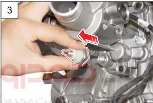
2. Turn the oil pressure switch (24 mm) anticlockwise.
