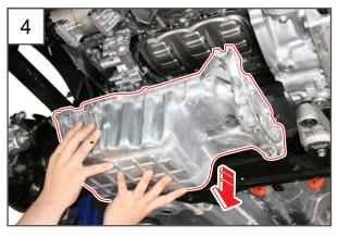
4. Remove the oil pan from the vehicle.
