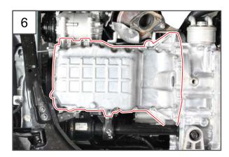
6. Unscrew the mounting bolts (A), (B), (C), and (D) for the oil pan from the underside of the engine assembly.
