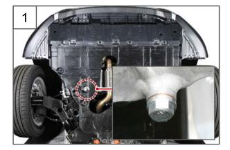
1. Unscrew the oil drain plug (14 mm) under the vehicle to drain the engine oil.
