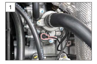
1. Disconnect the oil pressure switch connector from the underside of the thermostat.
