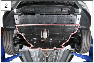
2. Remove the rear under cover under the vehicle.
