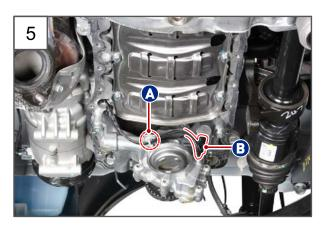
5. Disengage the VOP extension wiring clamp (A) and disconnect the VOP solenoid connector (B) from the oil pump.
