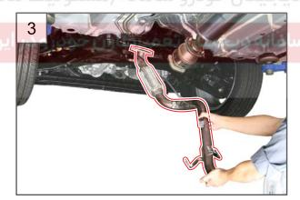
3. Remove the front exhaust pipe.
