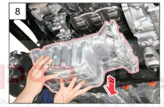
8. Remove the oil pan from the vehicle.
