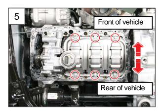
5. Unscrew the 6 mounting bolts (10 mm) for the baffle plate.
