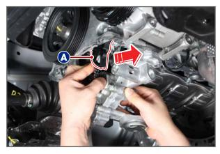
Install the oil pump to the oil pump chain after pulling the oil pump chain tensioner (A) in the direction of the arrow to release the tension of the oil pump chain.
