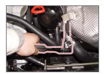
3. Remove the oil pressure switch.
