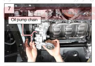
7. Separate the oil pump from the oil pump chain.
