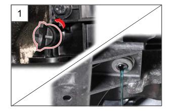
1. Drain the coolant. Refer to "COOLANT DRAIN AND FILL UP" under "REMOVAL AND INSTALLATION" subsection of "COOLING SYSTEM" section in "G16DF ENGINE" chapter.
